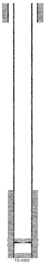
12-1/4" hole @ 382' 8-5/8" csg @ 382' w/ 200sx-TOC-Surf-Circ
