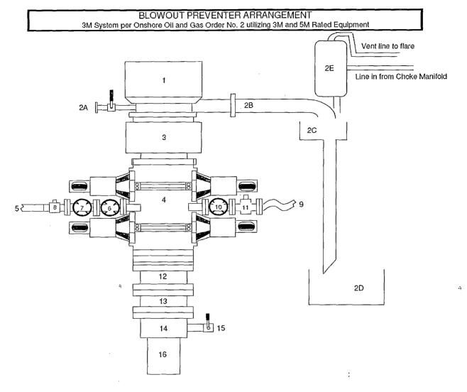
Description Item Rotating Head, 11" Fill up Line and Valve 2B Flow Line (10") 2C Shale Shakers and Solids Settling Tank 2D Cuttings Bins for Zero Discharge Rental Mud Gas Separator with vent line to flare and return line to mud system 2E Annular BOP (11", 3M)
