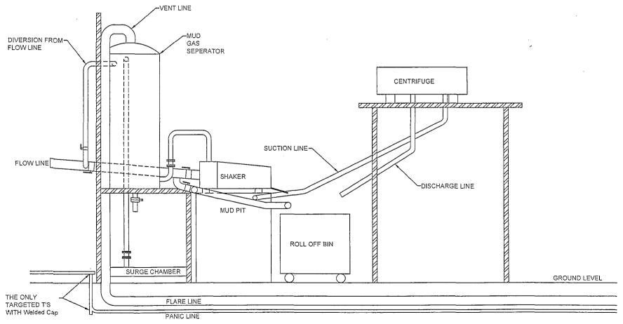
The flare discharge must be 100' from wellhead for non H2S wells and 150' from wellhead for wells expected to encounter H2S.
