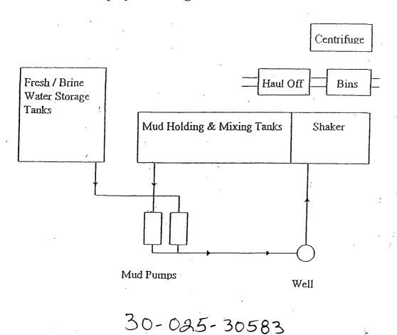
Closed Loop System Design & Construction
