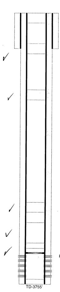
12-1/4" hole @ 501' 8-5/8" csg @ 501<u>'</u> w/ 350sx-TOC-Surf-Circ
