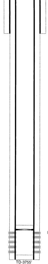
12-1/4" hole @ 501' 8-5/8" csg @ 501' w/ 350sx-TOC-Surf-Circ
