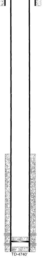
12-1/4" hole @ 295' 8-5/8" csg @ 295' w/ 175sx-TOC-Surf-Circ
