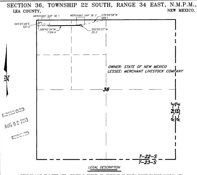
A STRIP OF LAND 30.0 FEET WIDE, LOCATED IN SECTION 36, TOWNSHIP 22 SOUTH, RANGE 34 EAST, N.M.P.M., LEA COUNTY, NEW MEXICO AND BEING 15.0 FEET LEFT AND RIGHT OF THE FOLLOWING DESCRIBED CENTERLINE SURVEY.
