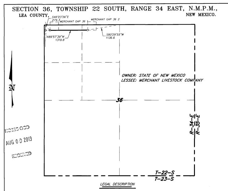
A STRIP OF LAND 30.0 FEET WIDE, LOCATED IN SECTION 36, TOWNSHIP 22 SOUTH, RANGE 34 EAST, N.M.P.M., LEA COUNTY, NEW MEXICO AND BEING 15.0 FEET LEFT AND RIGHT OF THE FOLLOWING DESCRIBED CENTERLINE SURVEY.
