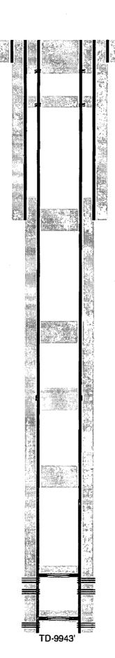
17-1/2" hole @ 354' 13-3/8" csg @ 354' w/ 375sx-TOC-Surf-Circ
