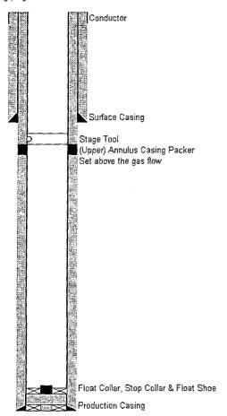
Two-Stage Cementing (Alternative for Oil / Water / Gas & Water Flow)
