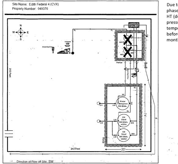
Due to High line pressure, we will add temporary 3 phase separator (denoted by blue square) to bypass the HT (denoted by the big X as bypassed). Once the line pressure is back to normal, we will remove the temporary separator and use existing facility. Like before. Expected duration of temporary solution is 6 months
