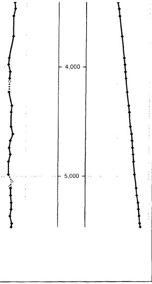
Inclination readings displayed in a small font were measured with slightly lower decoding accuracy than normal. This could occur, for example, if the Driller changed pump speed or tagged bottom prior to obtaining survey. These surveys are often very accurate. However, any such measurement that appears 'out of line' should be confirmed with a repeat survey.
