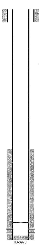
12-1/4" hole @ 270' 8-5/8" csg @ 267' w/ 200sx-TOC-Surf-Circ
