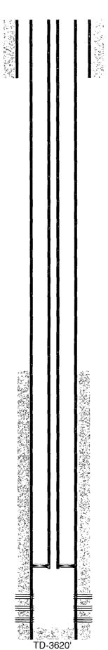
11" hole @ 349' 8-5/8" csg @ 349' w/ 300sx-TOC-Surf-Circ
