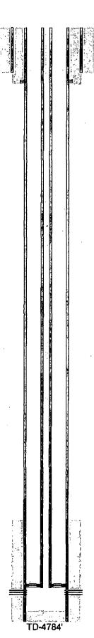
12-1/4" hole @ 392' 8-5/8" csg @ 392' w/ 325sx-TOC-Surf-Circ
