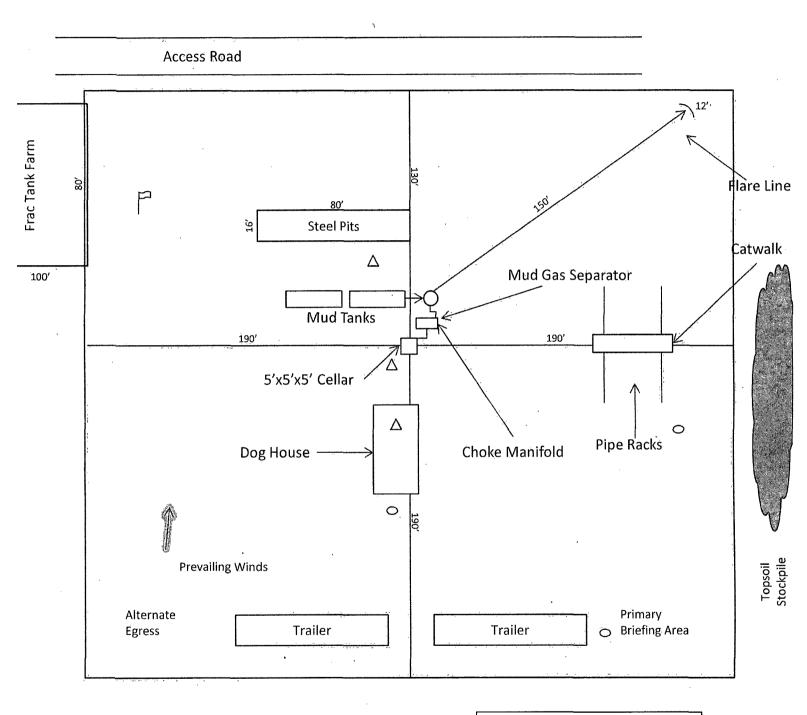
Exhibit D – Rig Diagram Ν Wind Direction Indicators P Cuervo Federal No. 21H (wind sock or streamers) Cimarex Energy Co. of Colorado H2S Monitors 14-23S-32E Δ. (alarms at bell nipple and shale SHL 330 FNL & 2310 FEL shaker) BHL 330 FSL & 2310 FEL 0 **Briefing Areas** Lea County, NM
