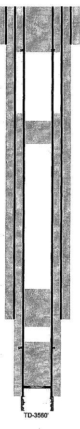
12-1/4" hole @ 360' 10-3/4" csg @ 360' w/ 250sx-TOC-Surf-Circ
