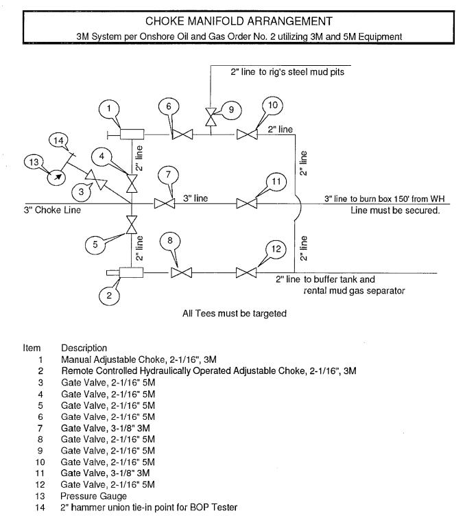
We will test each valve to 3000 psi from the upstream side.
