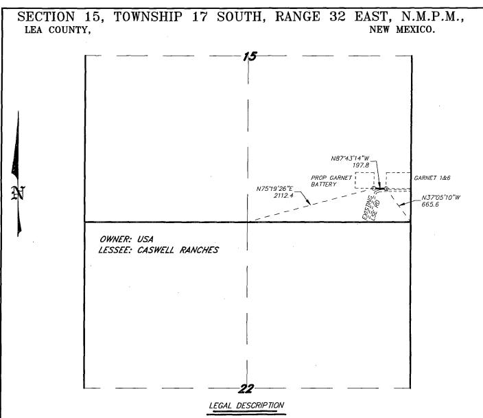
A STRIP OF LAND 30.0 FEET WIDE, LOCATED IN SECTION 15, TOWNSHIP 17 SOUTH, RANGE 32 EAST, N.M.P.M., LEA COUNTY, NEW MEXICO AND BEING 15.0 FEET LEFT AND RIGHT OF THE ABOVE PLATTED CENTERLINE SURVEY.
