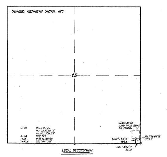
A STRIP OF LAND 30.0 FEET WIDE, LOCATED IN SECTION 15, TOWNSHIP 20 SOUTH, RANGE 34 EAST, N.M.P.M., LEA COUNTY, NEW MEXICO AND BEING 15.0 FEET LEFT AND RIGHT OF THE FOLLOWING DESCRIBED CENTERLINE SURVEY.
