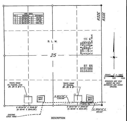
A strip of land, 30 feet in width, being 569.28 feet or 34.502 rods in length situated in Section 25, Township 23 South, Range 32 East, N. M. P. M., Lea County, New Mexico, being 15 feet left and 15 feet right of the following described survey of centerline across the land of the B. L. M.:
