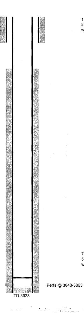
12-1/4" hole @ 375' 8-5/8" csg @ 375' w/ 300sx-TOC-Surf-Circ
