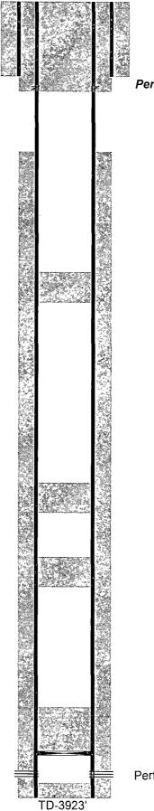
12-1/4" hole @ 375' 8-5/8" csg @ 375' w/ 300sx-TOC-Surf-Circ
