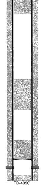
6-3/4" hole @ 4050' 4-1/2" csg @ 4043' w/ 630sx-TOC-Surf-Circ
