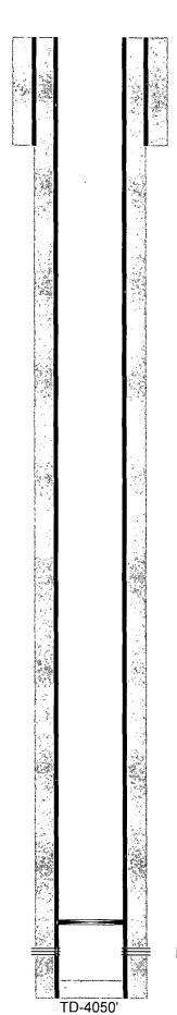
9-7/8" hole @ 463' 7-5/8" csg @ 458' w/ 200sx-TOC-Surf-Circ
