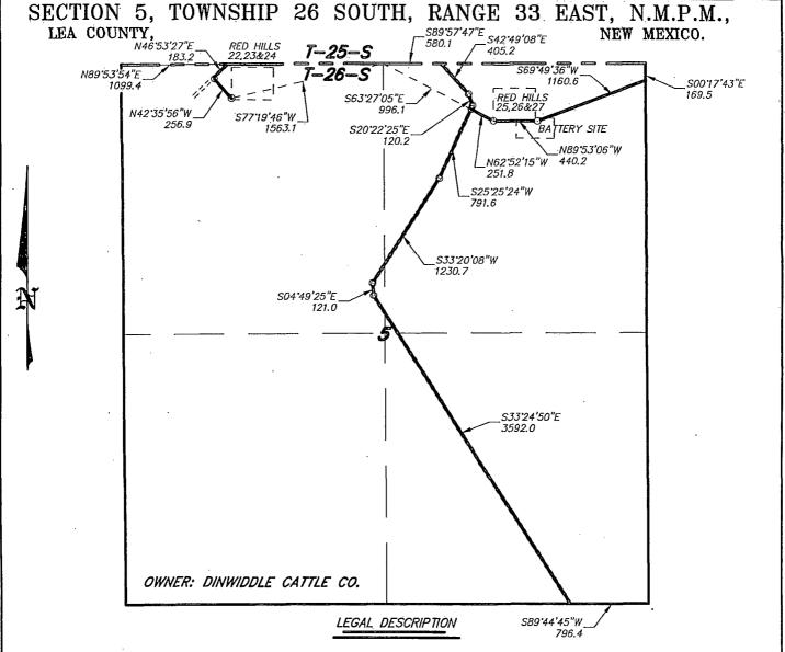
A STRIP OF LAND 30.0 FEET WIDE, LOCATED IN SECTION 5, TOWNSHIP 26 SOUTH, RANGE 33 EAST, N.M.P.M., LEA COUNTY, NEW MEXICO AND BEING 15.0 FEET LEFT AND RIGHT OF THE FOLLOWING DESCRIBED CENTERLINE SURVEY.
