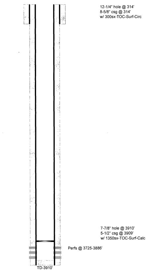
12-1/4" hole @ 314' 8-5/8" csg @ 314' w/ 300sx-TOC-Surf-Circ
