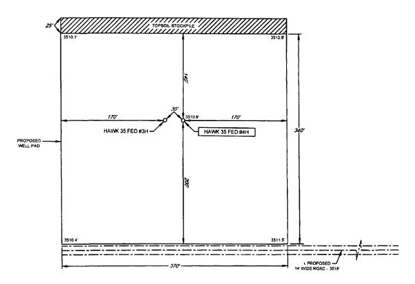
ALL BEARINGS, DISTANCES, AND COORDINATE VALUES CONTAINED HEREON ARE GRID BASED UPON THE NEW MEXICO STATE PLANE COORDINATE SYSTEM, EAST ZONE OF THE NORTH AMERICAN DATUM 1927, U.S. SURVEY FEET
