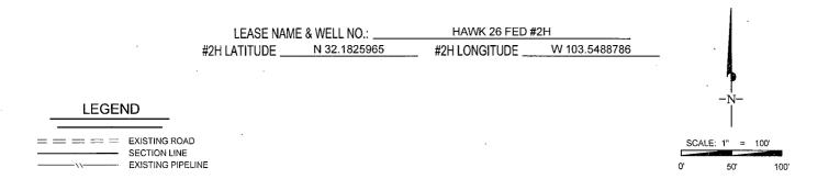
ALL BEARINGS, DISTANCES, AND COORDINATE VALUES CONTAINED HEREON ARE GRID BASED UPON THE NEW MEXICO STATE PLANE COORDINATE SYSTEM, EAST ZONE OF THE NORTH AMERICAN DATUM 1927, U.S. SURVEY FEET
