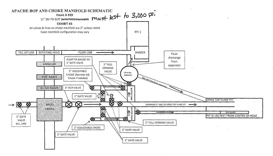
\*\*\* If H2S is encountered in quantities greater than 100ppm, Apache will shut in well & install a remote operated choke \*\*\*
