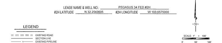
ALL BEARINGS, DISTANCES, AND COORDINATE VALUES CONTAINED HEREON ARE GRID BASED UPON THE NEW MEXICO STATE PLANE COORDINATE SYSTEM, EAST ZONE OF THE NORTH AMERICAN DATUM 1927, U.S. SURVEY FEET
