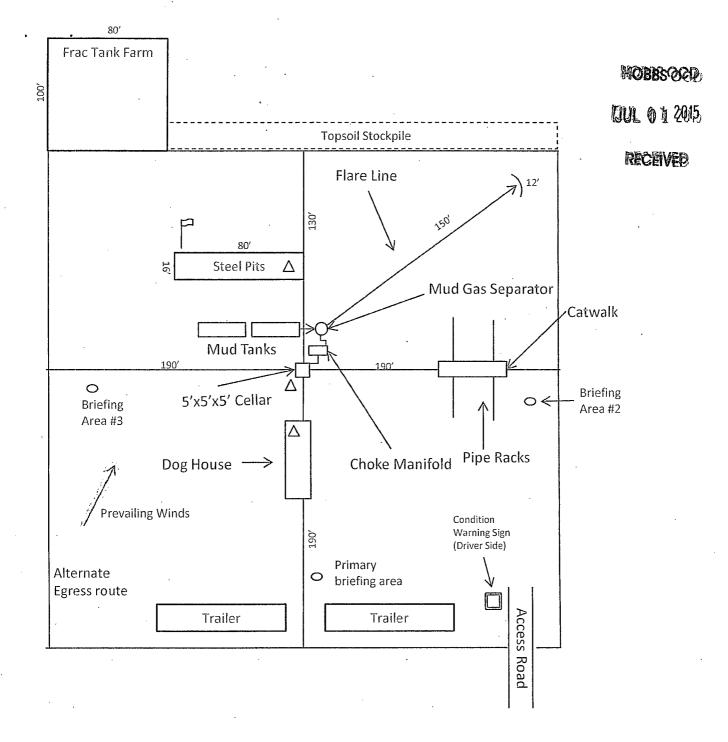
Ν Exhibit D – Rig Diagram Wind Direction Indicators Hallertau 5 Federal 5H (wind sock or streamers) Cimarex Energy Co. of Colorado 5-26S-32E H2S Monitors Δ (alarms at bell nipple and shale SHL 330' FSL & 480' FEL shaker) BHL 330' FNL & 940' FEL Lea County, NM 0 **Briefing Areas**
