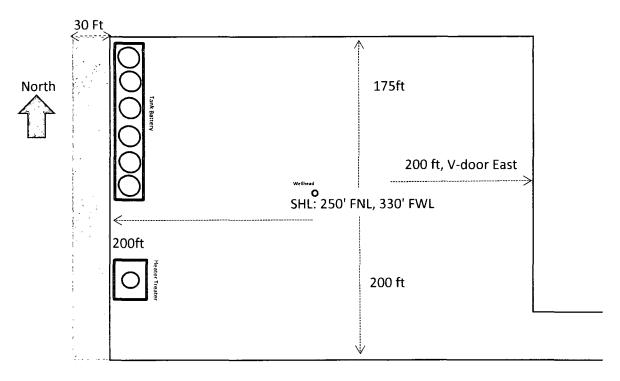
If well is found productive a tank battery will be constructed Battery will be burmed and lined approx. 3-500 bbls oil tanks & 3-500 bbl water tanks
