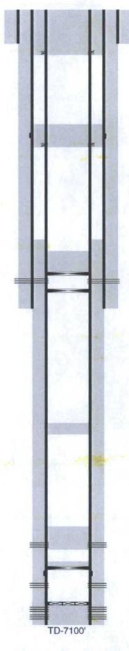
12-1/2" hole @ 3449' 9-5/8" csg @ 3449' DVT @ 1603' 1st w/ 928sx-TOC-1600'-Circ 2nd w/ 900sx-TOC-Surf-Circ
