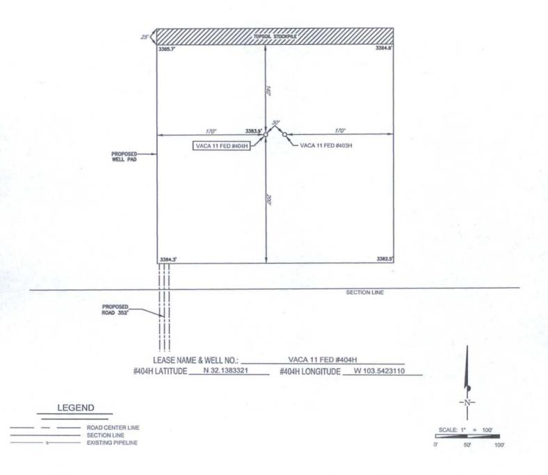
ALL BEARINGS, DISTANCES, AND COORDINATE VALUES CONTAINED HEREON ARE GRID BASED UPON THE NEW MEXICO STATE PLANE COORDINATE SYSTEM, EAST ZONE OF THE NORTH AMERICAN DATUM 1927, U.S. SURVEY FEET
