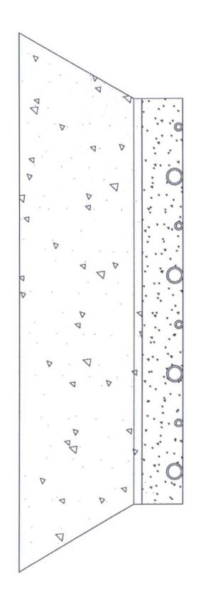
SOFT FILL DIRT OR SAND WITH NO ROCKS OR SOLID PARTICLES GREATER THAN 1" IN CIRCUMFERENCE FLOW LINE WILL BE 4" COATED STEEL PIPE w/ AN OPERATING PRESSURE UP TO 1480# PSI. GAS SUPPLY LINE WILL BE 2" STEEL PIPE w/ AN OPERATING PRESSURE UP TO 1100# PSI. BACKFILL DIRT TO BE AS FREE OF ROCKS AND LARGE PARTICLES AS POSSIBLE
