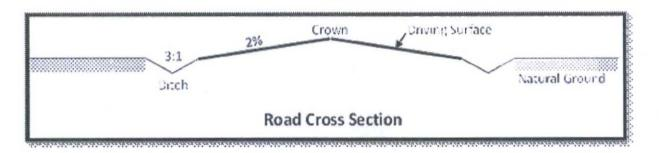
f. The access road will be constructed with a ditch on each side of the road.
