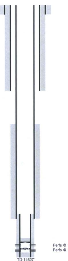
17-1/2" hole @ 727' 13-3/8" csg @ 727' w/ 575sx-TOC-Surf-Circ
