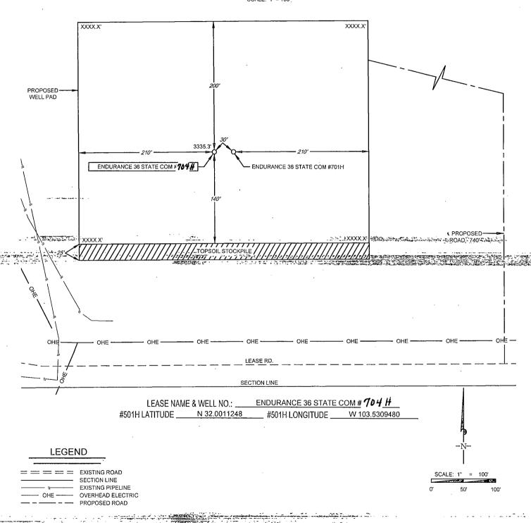
ALL BEARINGS, DISTANCES, AND COORDINATE VALUES CONTAINED HEREON ARE GRID  $\Box$  BASED UPON THE NEW MEXICO STATE PLANE COORDINATE SYSTEM; EAST ZONE OF THE NORTH AMERICAN DATUM 1927, U.S. SURVEY FEET
