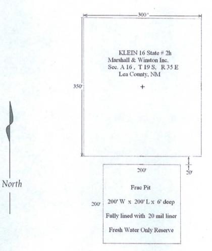
Diagram attachment to C-103, dated 12/17/2012, indicating the orientation of the Frac Pit (fresh water storage reserve) in relation to the well pad.
