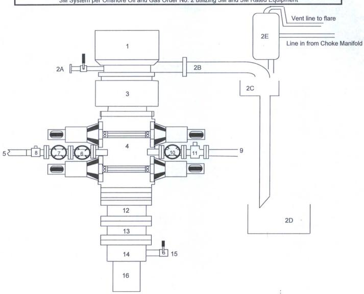
Item Description Rotating Head (11") 1 2A Fill up Line and Valve 2B Flow Line (8")
