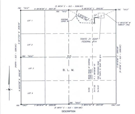
A strip of land 30 feet wide, being 519.57 feet or 31.489 rods in length lying in Section 31, Township 19 South, Range 33 East, N. M. P. M., Lea County, New Mexico, being 15 feet left and 15 feet right of the following described survey of a centerline across B. L. M.;
