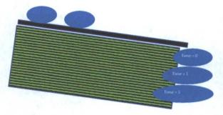
In the next figure, Time = 0 is about 15-20 years after closure. At Time=0, moisture that collected at the edge of the geomembrane cap begins to intrude into the heterogeneous stabilized cuttings, moving vertically and horizontally at a <u>maximum</u> expected ratio of 3 feet vertical to 1 foot horizontal. Time = 1 is about 20-25 years after closure and Time = 2 could be 27-32 years after closure, depending
