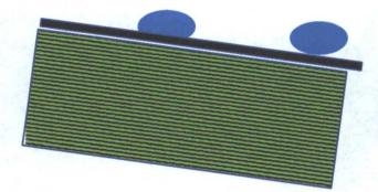
About 3-5 years after pit closure, the first pulse of moisture reaches the liner. After the next pulse of infiltration, about 7-15 years after closure, the moisture content of the dune sand immediately above the liner is sufficiently large that the moisture is expected to migrate down slope of the liner to the edge.
