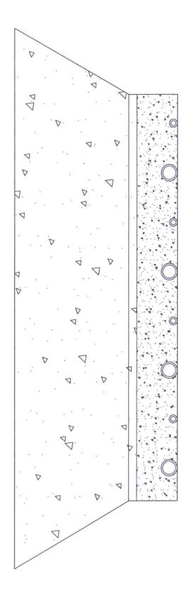
SOFT FILL DIRT OR SAND WITH NO ROCKS OR SOLID PARTICLES GREATER THAN 1" IN CIRCUMFERENCE FLOW LINE WILL BE 4" COATED STEEL PIPE w/ AN OPERATING PRESSURE UP TO 1480# PSI GAS SUPPLY LINE WILL BE 2" STEEL PIPE w/ AN OPERATING PRESSURE UP TO 1100# PSI. BACKFILL DIRT TO BE AS FREE OF ROCKS AND LARGE PARTICLES AS POSSIBLE
