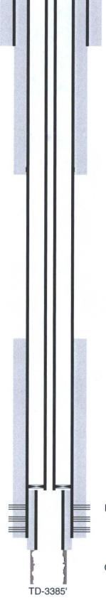
12-1/4" hole @ 472' 8-5/8" csg @ 472' w/ 250sx-TOC-Surf-Circ
