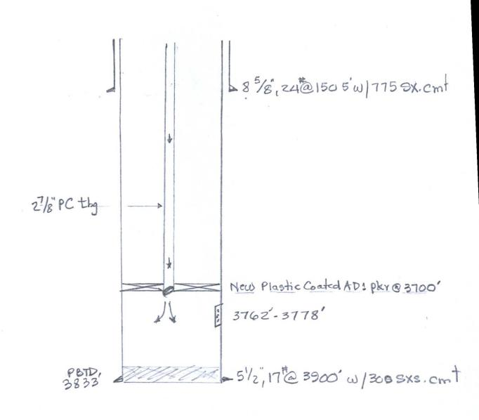
1- Found hole in 83rd it of tubing. 2. Replaced total 10 its PC Pipe w/ PC ADI-New PKX
