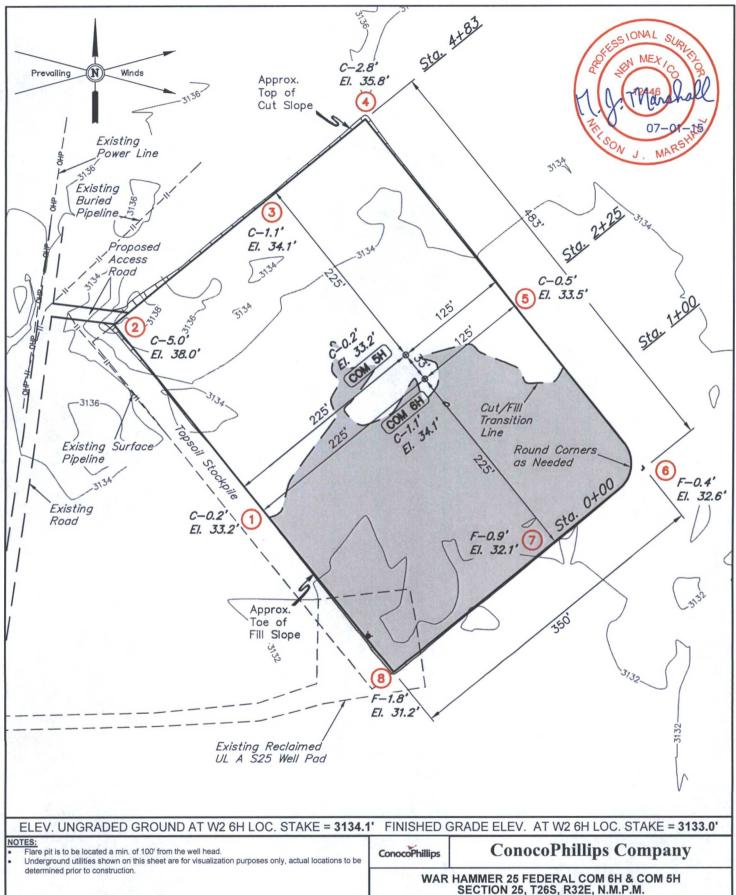
WAR HAMMER 25 FEDERAL COM 6H & COM 5H SECTION 25, T26S, R32E, N.M.P.M. NE 1/4 NE 1/4
