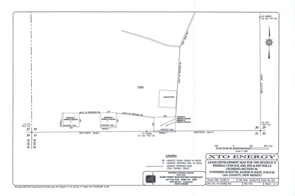
ROAD LEASE S86°41'29"E 400.0' 400.0' 400.0' 3"15'91'S FACILITY SITE W"15'91°503 3.67 AC. BURIED PIPELINE P.O.B. N86°40'29"W 400.0 N00'34'04 W 564.4' (TIE) 29 30 1/4 CORNER 281.1' (TIE) N89'25'56"E 2360.1 31 32 U.S. GLO B.C. "1912" U.S. GLO B.C. "1912"
