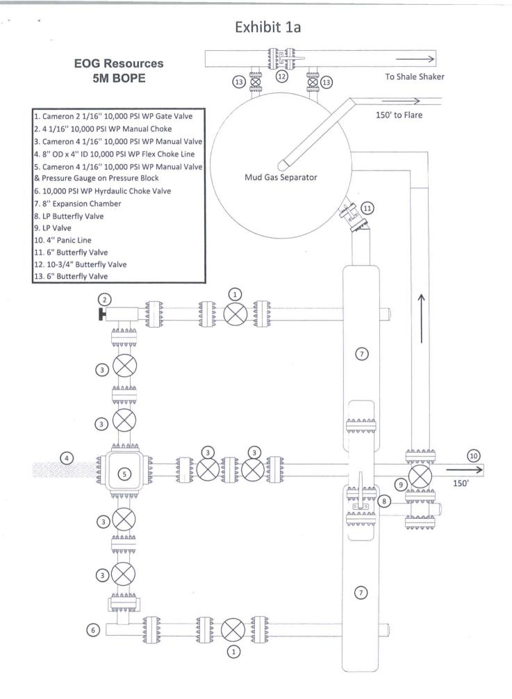
EOG 5M Choke Manifold Diagram (rev. 3/21/14)
