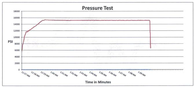
Test Pressure 15000 PSI Time Held at Test Pressure
