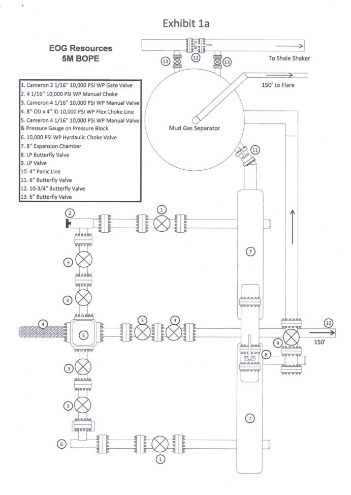
EOG 5M Choke Manifold Diagram (rev. 3/21/14)
