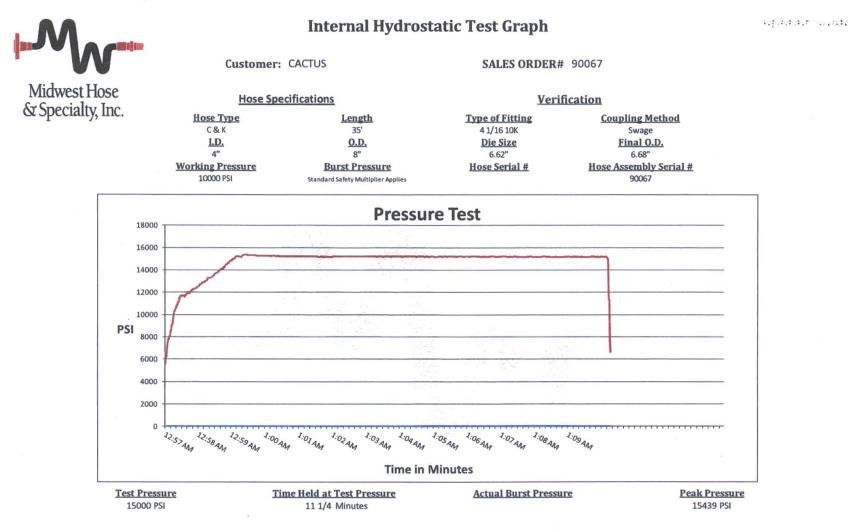
Comments: Hose assembly pressure tested with water at ambient temperature.
