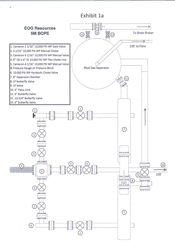
EOG 5M Choke Manifold Diagram (rev. 3/21/14)
