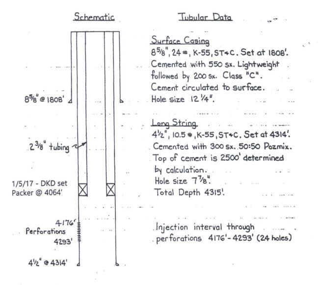
Tubing size is  $2^{3}8''$  which will be lined with a powered epoxy coating (Tuboscope TK-75 coating). Tubing will be set in a Baker AD-1 tension packer.
